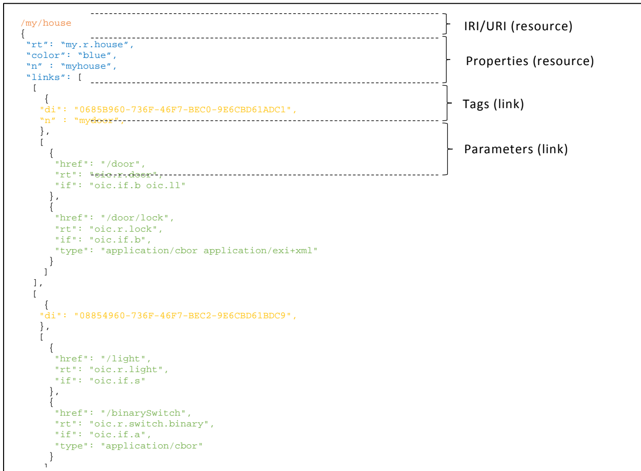
1318 1319 Figure 11: Example showing parts of OIC Collection and OIC Links
