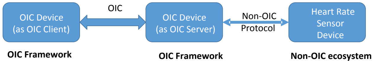
Figure 6: OIC Server bridging to Non-OIC device
